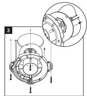
Secure to ceiling using suitable screws first making sure backdraught shutters are removed but shutter spider is left in position. Wire fan (See wiring details).
