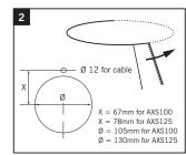
Cut an opening through the ceiling for the fan and electrical cable.
