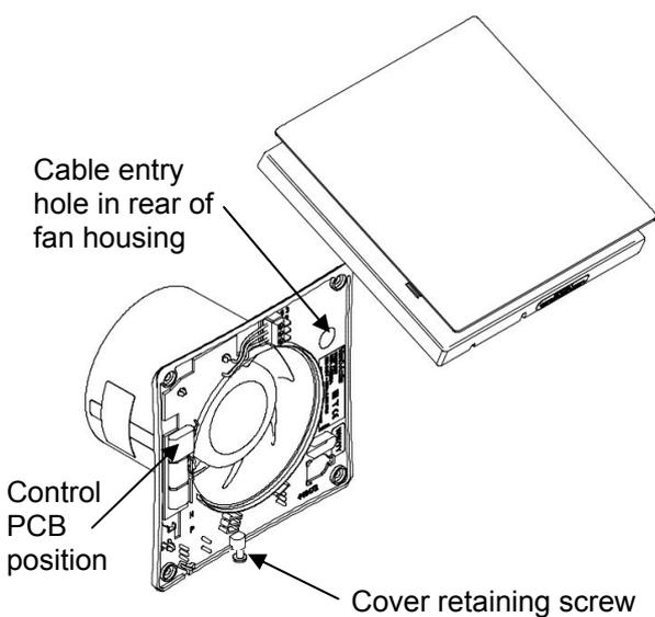
To remove the outer cover slide the cover to the right to release the 4 clips (1), then out towards you (2). To refit the cover, line up the 4 clips on the rear of the cover and slide to the left until you hear a "click".
